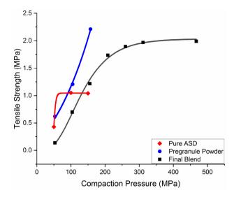
Fig. 3 Tabletability of powders in different stages of tablet formulation design, 70% POS-HPMCAS ASD (red), pregranulation blend (blue), and final blend (black). Lines were obtained by fitting the data to the Vreeman-Sun tabletability equation.
