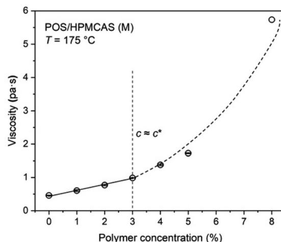
**Fig. 1** Viscosity-composition diagram of POS/HPMCAS at 175 °C.
