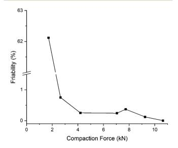
Fig. 6 Tablet friability profile of the final blend.
