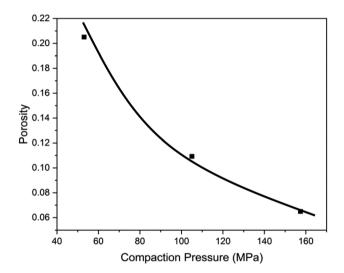
Fig. 4 Compressibility profile of the pre-granulation blend. The line was obtained by curve fitting with the Kuentz and Leuenberger (KL) equation.
