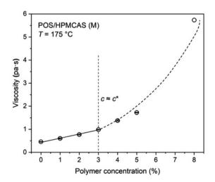
Fig. 1 Viscosity-composition diagram of POS/HPMCAS at 175 °C
