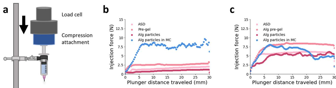
**Fig. 4** (a) Schematic of injection force testing set-up. Injection force (N) versus distance traveled by syringe plunger (mm) for formulations tested at (b)  $25\text{ }\mu\text{L s}^{-1}$  ( $\sim 1.3\text{ mm s}^{-1}$ ) and (c)  $150\text{ }\mu\text{L s}^{-1}$  ( $\sim 8.3\text{ mm s}^{-1}$ ).
