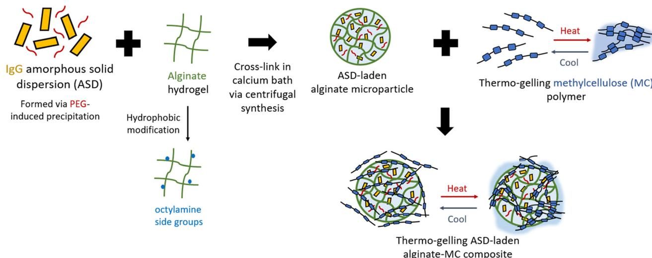
**Fig. 1** Conceptual schematic of the proposed dual-network hydrogel design, composing high-concentration antibody-loaded alginate microparticles with thermogelling methylcellulose polymer to result in a thermo-gelling composite hydrogel with complex inter-network interactions.
