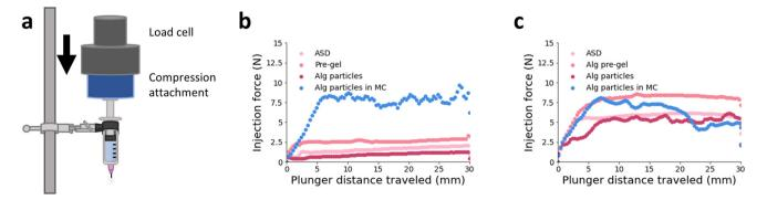
Fig. 4 (a) Schematic of injection force testing set-up. Injection force (N) versus distance traveled by syringe plunger (mm) for formulations tested at (b) 25  $\mu$ L s<sup>-1</sup> (~1.3 mm s<sup>-1</sup>) and (c) 150  $\mu$ L s<sup>-1</sup> (~8.3 mm s<sup>-1</sup>).
