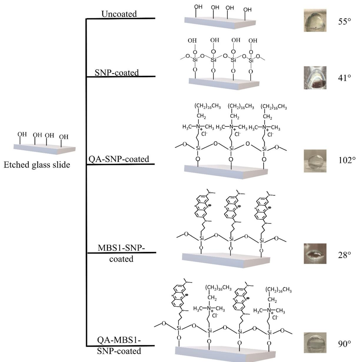
**Fig. 2** Schematic illustration of uncoated, SNP, QA-SNP, MBS1-SNP, and QA-MBS1-SNP coated glass surfaces and respective water contact angle measurements. QA-SNP and QA-MBS1-SNP coated surfaces showed water contact angle  $\geq 90^\circ$ , indicating hydrophobic surfaces.
