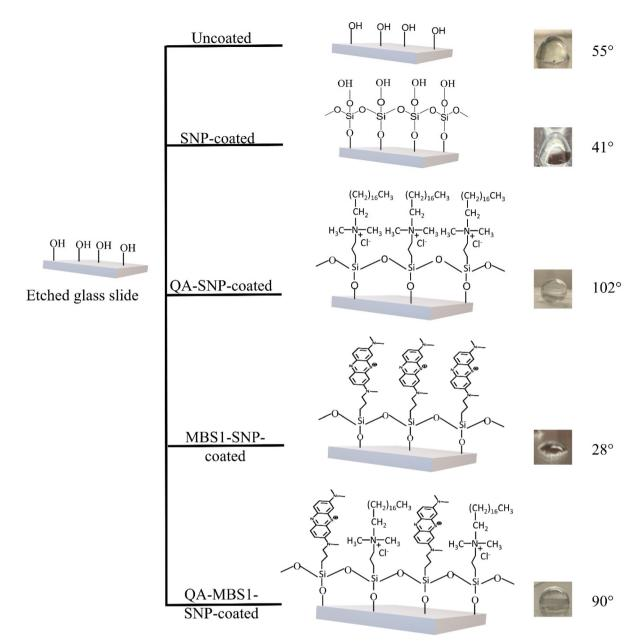
Fig. 2 Schematic illustration of uncoated, SNP, QA-SNP, MBS1-SNP, and QA-MBS1-SNP coated glass surfaces and respective water contact angle measurements. QA-SNP and QA-MBS1-SNP coated surfaces showed water contact angle ≥90°, indicating hydrophobic surfaces.
