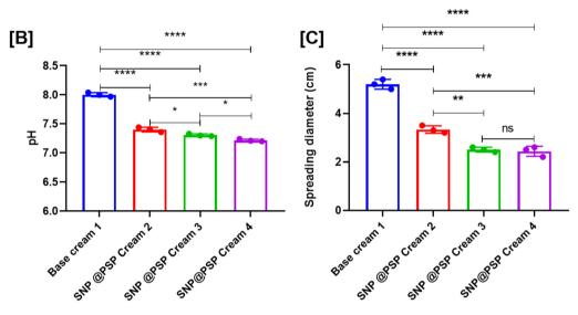
Fig. 1 (A) Base cream and SNP@PSP cream formulations; (B) pH values of formulated creams (n = 3); and (C) graphical representations of cream spreading diameter (n = 3).
