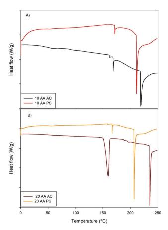
Fig. 4 Differential scanning calorimetry (DSC) thermograms of SP-A: (A) 10-AA and SP-A (B) 20-AA Peptides. (Exothermic peak is up. Endothermic peak is down). (N = 3).
