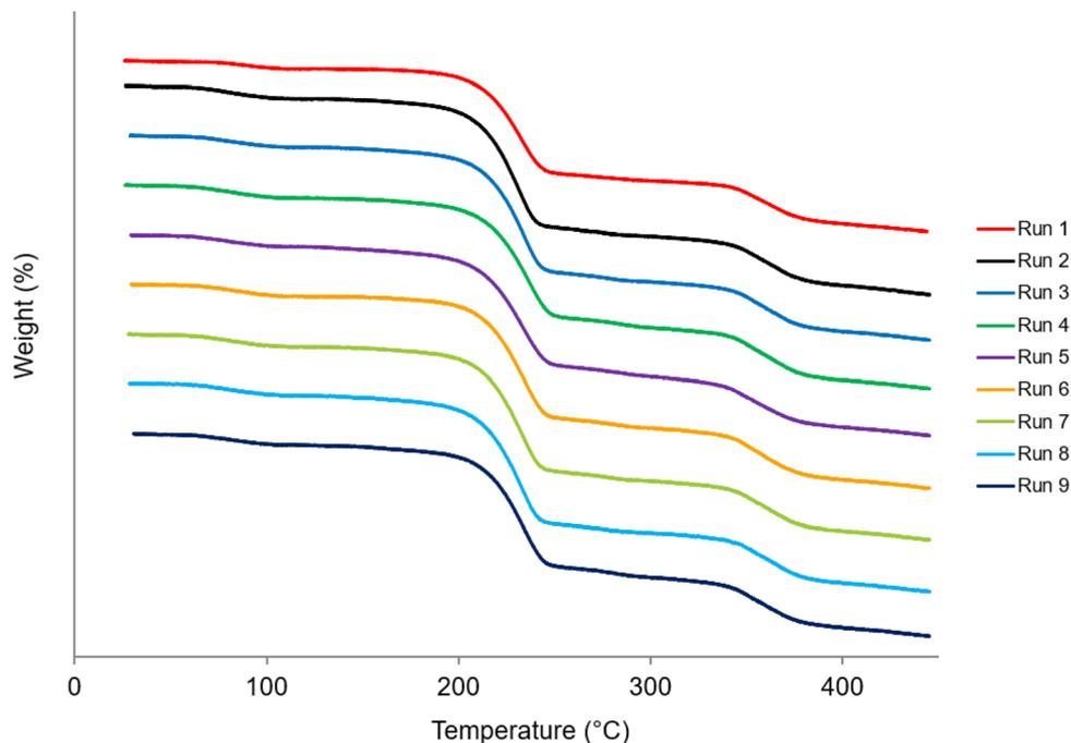
Fig. 7 TGA thermograms of Runs 1–9 at Day 0.
