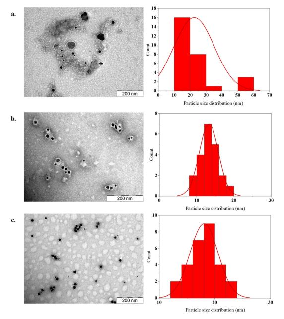
Fig. 5 TEM images and size distributions of the selected AuNPs for uptake and silencing study: (a) AuNP-W2R4, (b) AuNP-W3R3 and (c) AuNP-W4R4 (scale = 200 nm).
