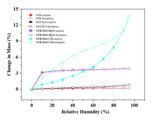
Fig. 8 Water sorption/desorption isotherms of GTB, DAS·H<sub>2</sub>O GTB-DAS-2H2O and GTB-DAS CM.
