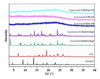
Fig. 1 PXRD patterns of GTB-DAS-2H<sub>2</sub>O and starting components, as well as GTB-DAS CM, GTB AM and DAS AM.
