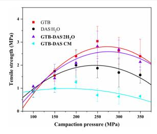
Fig. 9 Tabletability profiles of GTB, DAS·H<sub>2</sub>O, GTB-DAS·2H<sub>2</sub>O and **GTB-DAS CM**
