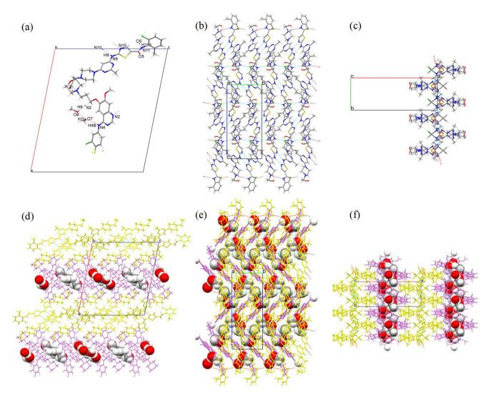
Fig. 4 (a) Asymmetric unit along the *b*-axis. DAS layer packed along (b) the *a*-axis and (c) the *c*-axis. 3D framework packed along (d) the *b*-axis, (e) the *a*-axis and (f) the *c*-axis for **GTB-DAS-2MeOH**. Violet molecules correspond to GTB, and yellow molecules correspond to DAS.
