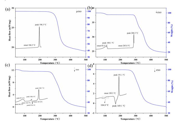
Fig. 2 TG and DSC thermograms of (a) GTB, (b) DAS·H<sub>2</sub>O, (c) GTB-DAS·2H<sub>2</sub>O and (d) GTB-DAS CM.
