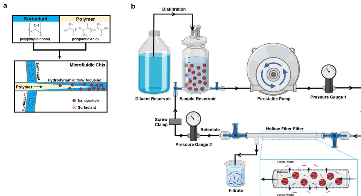
**Fig. 1** Schematic representation of the nanoparticle synthesis and purification. (a) Formulation of PLA–PVA nanoparticles using a flow focusing microfluidic device. (b) Schematic of the hollow fiber tangential flow filtration (TFF) system utilized for the purification of nanoparticles, shown under diafiltration. Figures were made using BioRender (<https://www.biorender.com/>).
