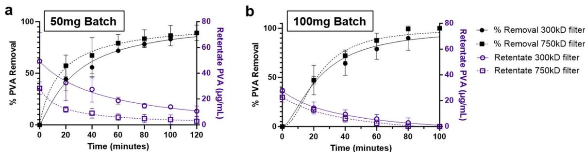
**Fig. 3** TFF PVA removal time-course. Quantified % PVA removal (black) and remaining PVA weight (blue) for (a) 50 mg and (b) 100 mg batches of PLA–PVA nanoparticles purified by TFF (300 kD and 750 kD filters).
