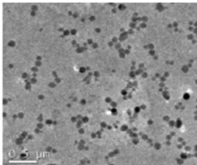
**Fig. 2** Cryo-TEM image of the spherical polymeric micelles. Shown is the P3S formulation which is assembled with a hydrophilic sulfobetaine to lipophilic BMA ratio of 50 : 50.
