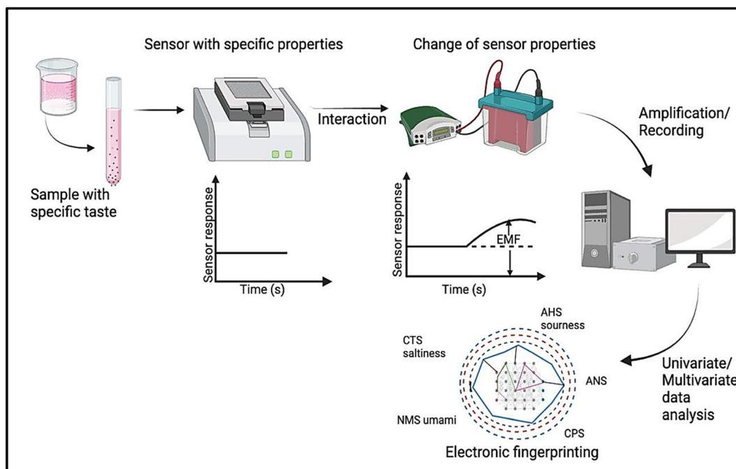
Fig. 5 Schematic representation of an electronic taste conveying system for identifying the degree of taste masking.<sup>188</sup>
