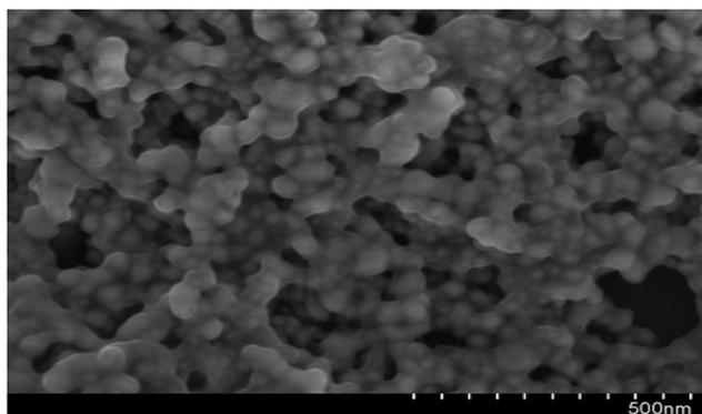
Fig. 8 FE-SEM images of CA-AgNPs at 500 nm magnification.
