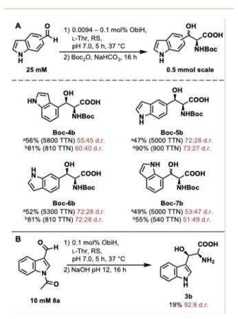
Fig. 4 Preparative-scale synthesis of (A) C4-C7 substituted and (B) C3 substituted β-OH L-Trp regioisomers. Product purity and dr was assessed via <sup>1</sup>H NMR. <sup>a</sup> The reaction was performed with ~0.1 mol% ObiH.  $^b$  The reaction was performed with  $\sim$ 0.01 mol% ObiH.
