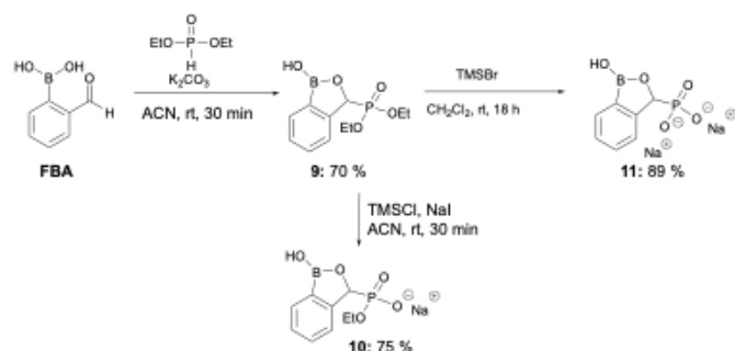
Figure 4. Synthesis of benzoxaborole derivatives containing a phosphorus(V) functionality.
