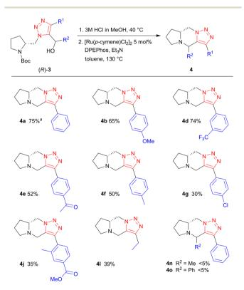
Scheme 4 Formation of fused triazole piperazines 4. Reagents and conditions: (1) 3 M HCl in MeOH, 40 °C, 1 h; (2)  $[Ru(p\text{-cymene})Cl_2]_2$  (5 mol%), DPEphos (10 mol%), Et<sub>3</sub>N (10 mol%), toluene, 130 °C, 24–48 h. Isolated yields for the 2-step process. <sup>a</sup> The corresponding enantiomer (*S*)-4a was also prepared in 58% yield from (*S*)-3a.
