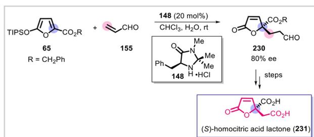
**Scheme 56** Organocatalyzed synthesis of a butenolide intermediate en route to (*S*)-homocitric acid lactone.
