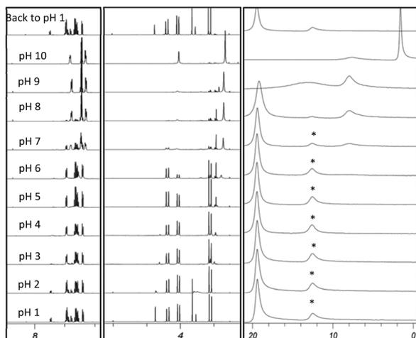
Fig. 3 <sup>1</sup>H and <sup>11</sup>B NMR data for 1 (full spectra available in SI). Left box: <sup>1</sup>H NMR aromatic region; middle box: <sup>1</sup>H NMR aliphatic region; right box <sup>11</sup>B NMR. \*The peak at ~13 ppm in the <sup>11</sup>B NMR is boric acid.
