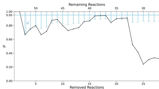
**Fig. 11** Fraction  $p$  of experimental rate constants for removed reactions falling in the confidence interval. Error bars represent the uncertainty  $\sigma$  in the 95% interval according to eqn (9).
