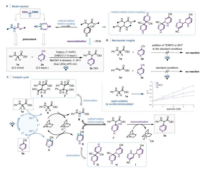
Scheme 2 (A) Model reaction in the radical-radical hetero-coupling of two captodative radials. (B) Mechanistic studies. (C) Proposed reaction mechanism
