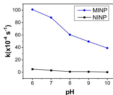
**Fig. 1** Dependence of acetal hydrolysis of S1 catalyzed by MINP<sub>1</sub> versus NINP at 40 °C. [S1] = 100  $\mu\text{M}$ . [MINP<sub>1</sub>] = [NINP] = 5.0  $\mu\text{M}$ .
