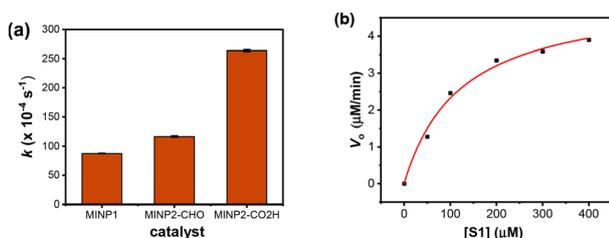
**Fig. 2** (a) Comparison of the rate of hydrolysis of **S1** at pH 7 catalyzed by different MINPs at 40 °C in 10 mM HEPES buffer. [**S1**] = 100  $\mu$ M. [MINP] = 5.0  $\mu$ M. (b) Michaelis–Menten plot for the hydrolysis of substrate **S1** by MINP<sub>2</sub>-CO<sub>2</sub>H in a 10 mM HEPES buffer (pH 7.0) at 40 °C.
