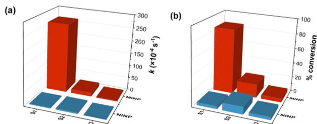
**Fig. 3** (a) Substrate selectivity of MINP<sub>2</sub>-CO<sub>2</sub>H in the catalytic hydrolysis of S1–3. The reaction rate was monitored by UV at 40 °C in a 10 mM HEPES buffer at pH 7.0. (b) Selectivity of MINP<sub>2</sub>-CO<sub>2</sub>H in the catalytic hydrolysis of an equimolar mixture of S1–3. Reactions were performed in duplicate at 40 °C for 4 h in 10 mM HEPES buffer at pH 7.0. Dibromomethane was used as an internal standard. [S1] = [S2] = [S3] = 2.0 mM. [MINP] = 0.10 mM.
