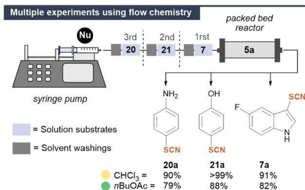
Fig. 2 Multiple consecutive experiments using flow chemistry. See the ESI† for details. Color code; volatile organic compound-VOC (yellow) and environmentally friendly solvent (green).
