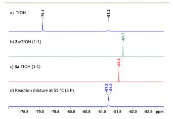
Fig. 2  $^{19}$ Ft<sup>1</sup>H} NMR analysis (the -78 to -83 ppm region was zoomed for clarity;  $C_6F_6$  was used as a reference at -165 ppm) of TfOH along with Fmoc-NH $_2$  (2a), the hydroamination product (3a) and the reaction mixture after 5 h. For detailed reaction conditions and analysis, see the ESI.†
