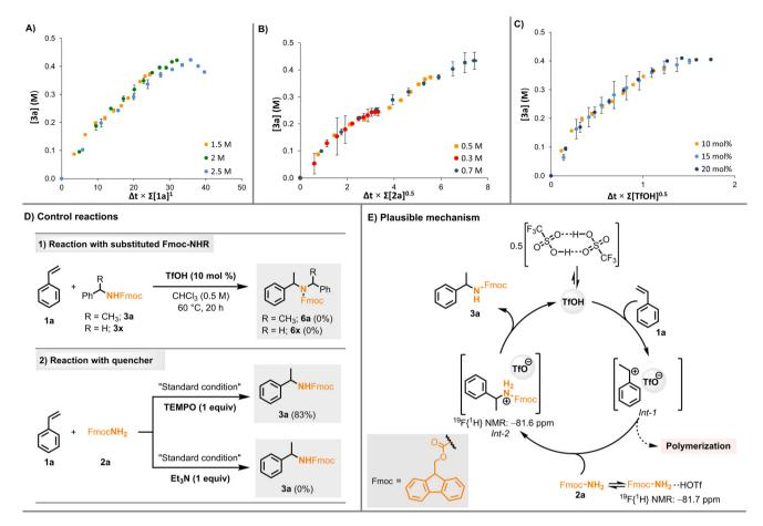
Fig. 3 VTNA plot of (A) styrene; (B) Fmoc-NH2; and (C) TfOH (standard deviations are for two independent experiments). (D) Control reaction; standard conditions: styrene (3 equiv.), Fmoc-NH2 (1 equiv.), TfOH (10 mol%), CHCl3 (0.5 M), 60 °C, 5 h. (E) Plausible mechanism.
