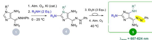
**Scheme 1** (A) Classical arylazoimidazole synthesis still used; (B) previously developed pathway for the synthesis of arylazoimidazoles **3** from amidrazone-based imidazole precursors **1**; (C) and synthesis of the new arylazoimidazoles **5** here presented.
