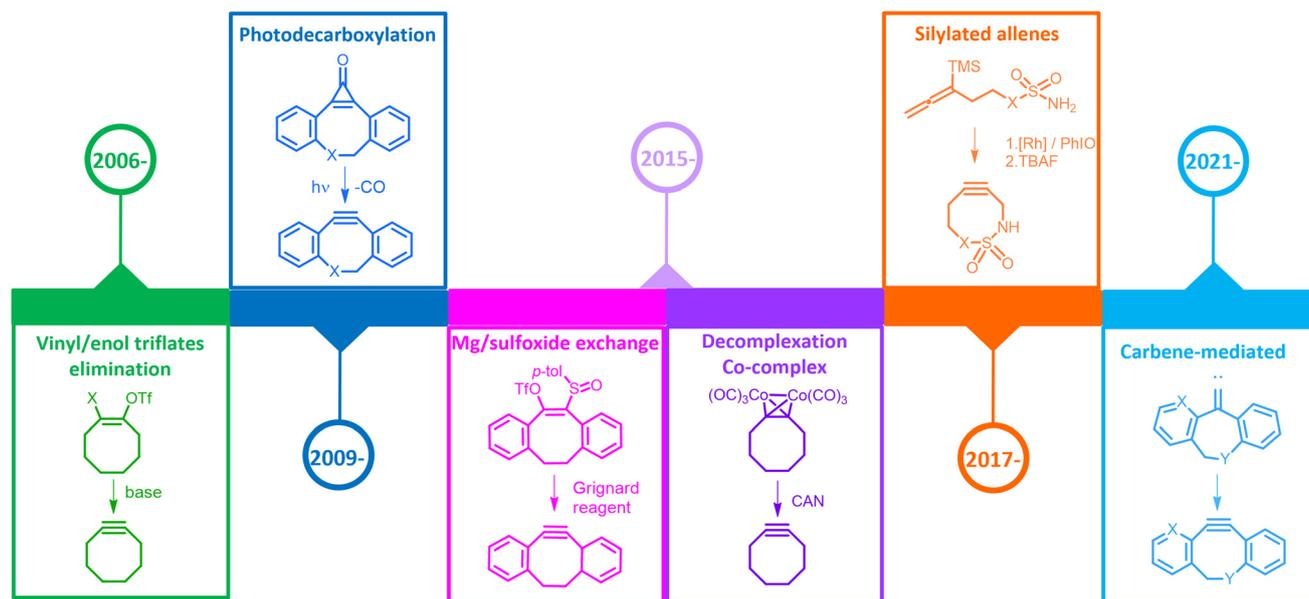
Fig. 1 Timeline of synthetic methodologies applied to cyclooctyne synthesis.
