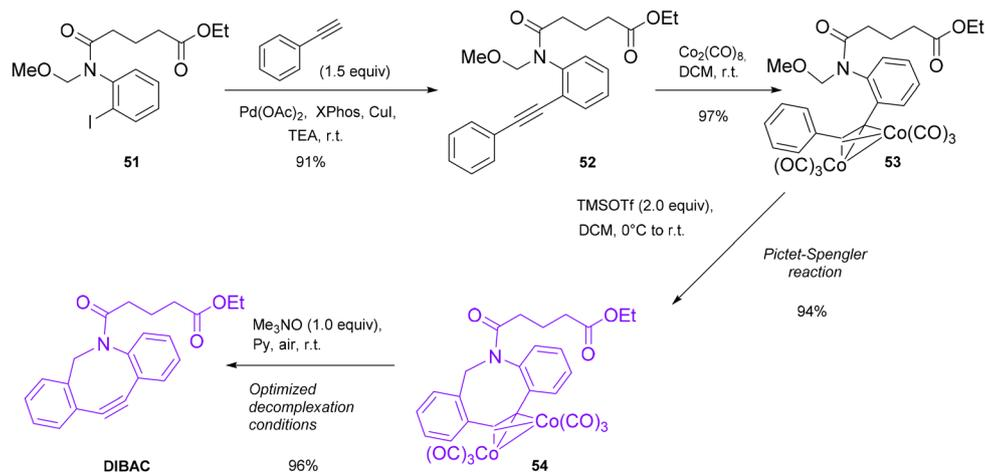
**Scheme 14** DIBAC synthesis using the Co-complex decomplexation methodology.
