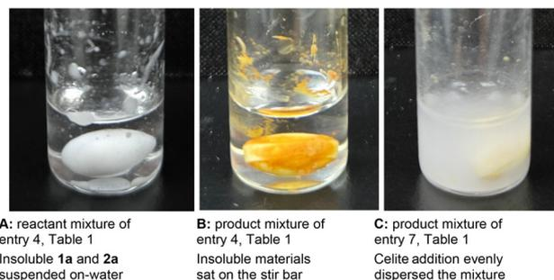
Fig. 1 The effect of Celite as dispersant.
