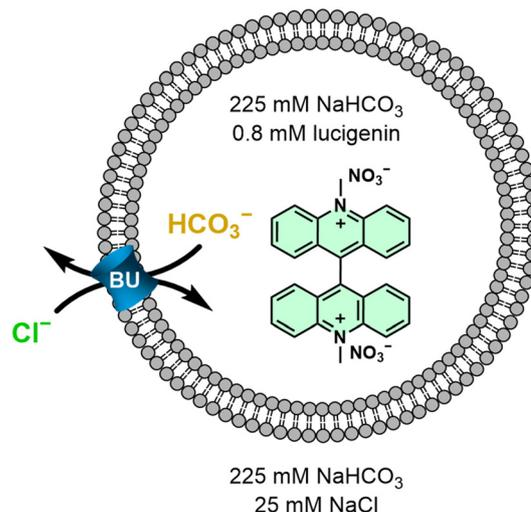
**Fig. 4** Schematic representation of the lucigenin assay.
