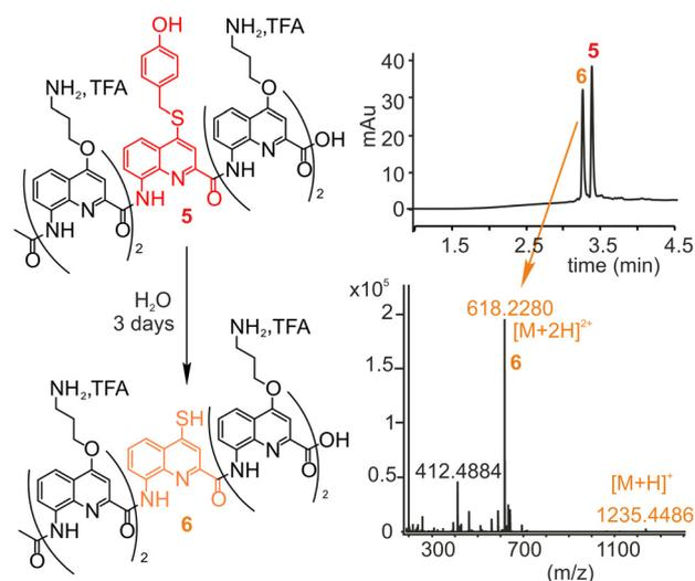
**Fig. 3** Monitoring of the *para*-hydroxybenzyl side-chain elimination of  $Q^U$  in pure water on model pentamer **5**. The formation of the 4-mercapto-quinoline-containing pentamer **6** was confirmed by LC-MS analysis.
