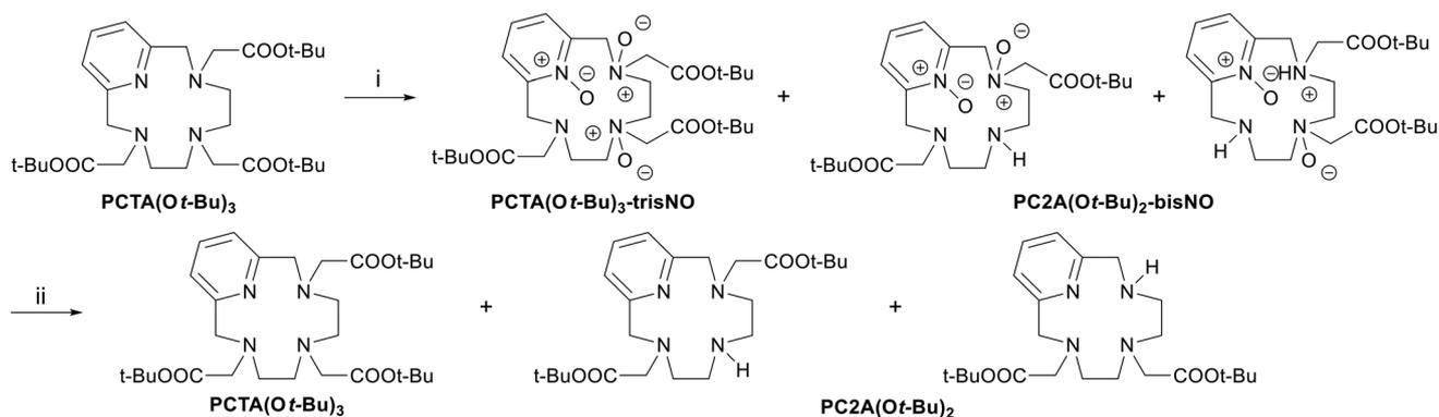
**Scheme 6** Observed products upon reaction between PCTA(Ot-Bu)<sub>3</sub> and mCPBA and successive treatment with Na<sub>2</sub>SO<sub>3</sub>. (i) mCPBA (3–6 equiv.), DCM, rt, 1 h; (ii) Na<sub>2</sub>SO<sub>3</sub> (5 equiv.), H<sub>2</sub>O, rt, overnight.
