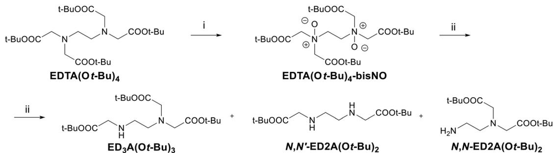
**Scheme 3** Dealkylation reaction on EDTA(Ot-Bu)<sub>4</sub>. (i) mCPBA, DCM, rt, 1–5 h; (ii) FeCl<sub>2</sub>, DCM, rt, 1 h.
