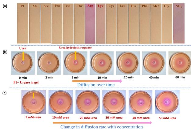
**Fig. 4** Demonstration of visual detection of (a) amino acids (as 5 mM aqueous solution) and ammonia (as fumes) using **P1** dip-coated paper strips; (b) ammonia formation during diffusion of 60 mM urea (under enzymatic hydrolysis) over time; and (c) ammonia formation and change in the diffusion area as the urea concentration changes from 5 to 50 mM (after 60 minutes; agarose gel containing **P1** (40  $\mu M$ ) + urease (20 nM)).
