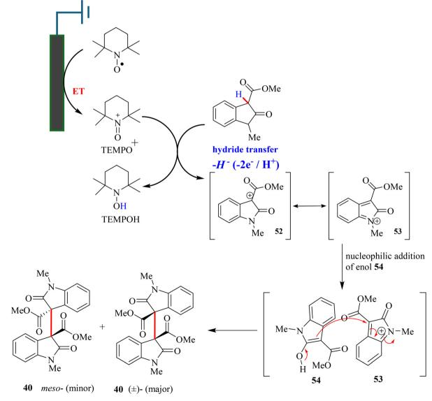
Scheme 13 TEMPO-catalyzed electro-oxidative dimerization of 3-carboxylate-2-oxindole.
