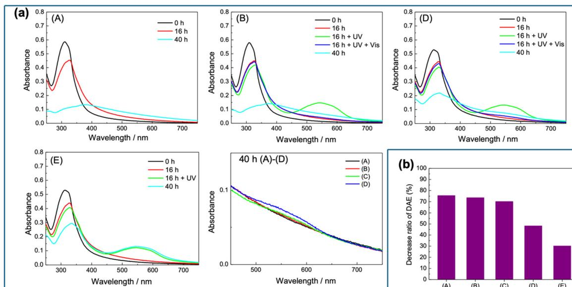
**Fig. 4** UV-vis absorption spectra of DNA–DAE solutions (D-PBS/DMSO = 95 : 5 (v/v), DNA: 75.8  $\mu$ Mbp, and DAE: 25  $\mu$ M) at various stages of light irradiation and time lapse schedules of conditions (A)–(E) (a) and the decrease ratio of DAE (loss from the solution due to precipitation) under different irradiation conditions (b).
