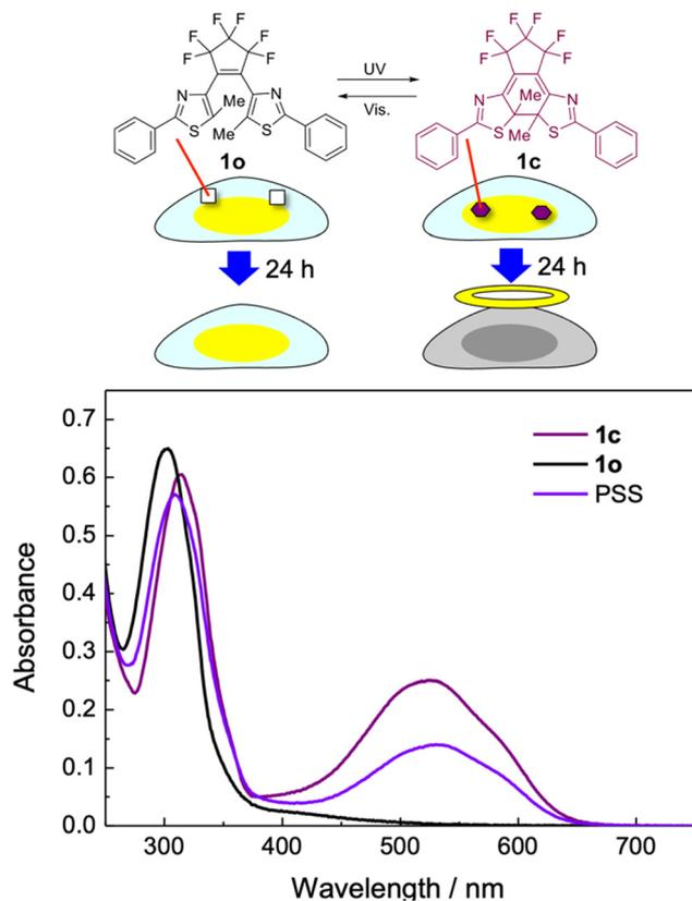
**Fig. 1** Chemical structures and the effect on cell culture of **1o** and **1c** (a) and UV-vis absorption spectra of **1o**, **1c** in a solution (b, D-PBS : DMSO = 95 : 5 and DAE concentration = 25  $\mu$ M) and the photostationary state (PSS, **1o** : **1c** = 44.5 : 55.5) under UV irradiation at 365 nm (b).
