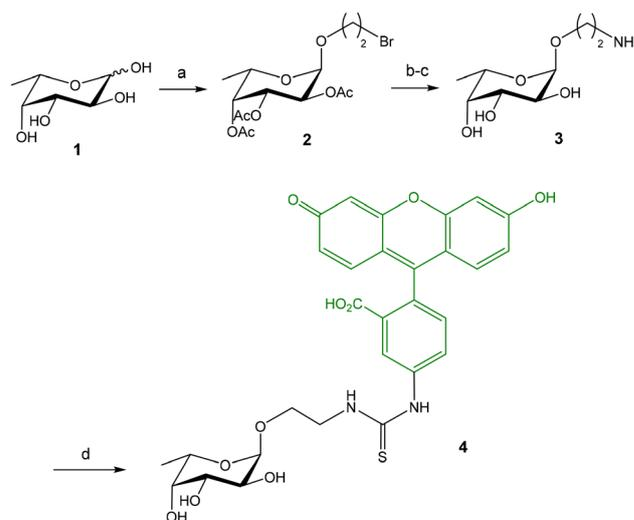
**Fig. 3** Synthesis of fluorescein-labeled fucoside probe **4**. Reagents and conditions: (a)  $\text{La}(\text{OTf})_3$ , 2-bromoethanol, 70 °C;  $\text{Ac}_2\text{O}$ , Py, 46%; (b)  $\text{NaN}_3$ , DMF, 70 °C, 70%; (c)  $\text{NaOMe}$ , MeOH;  $\text{H}_2$ , Pd/C, EtOH, 66%; (d) FITC,  $\text{NaHCO}_3$ , DMF, 96%.
