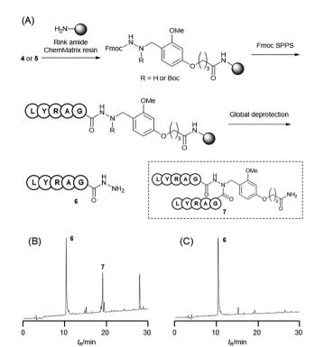
Fig. 3 (A) Solid-phase peptide synthesis using linker 4 or 5. UV trace of a crude peptide synthesized using linker 4 (B) and linker 5 (C). Global deprotection conditions: TFA-TIS- $H_2O = 95 : 2.5 : 2.5 (v/v)$  at 37 °C for 2 h.
