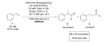
Fig. 2 Hydroformylation of styrene (1) in aqueous medium using the surfactant Triton X-100, with the following additives necessary for the enzymatic transamination: 250 mM L-alanine, 150 mM D-glucose and ammonium formate, 1 mM NADH and PLP, and sterile crude extract of empty vector Escherichia coli BL21-(DE3) (30%, v/v).
