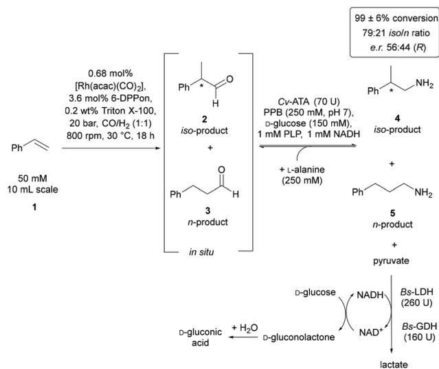
**Fig. 5** Chemoenzymatic synthesis of the primary amines 2-phenylpropan-1-amine (**4**) and 3-phenylpropan-1-amine (**5**) starting from styrene (**1**). A 6-DPPon/rhodium-catalysed hydroformylation of styrene (**1**) applying an aqueous solution utilizing the surfactant Triton X-100 was combined with Cv-ATA catalysed enzymatic transamination of the *in situ*-formed aldehydes.
