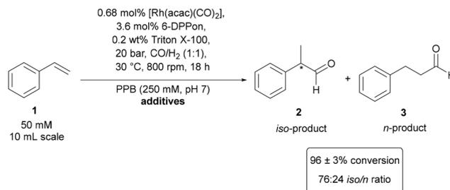
**Fig. 2** Hydroformylation of styrene (**1**) in aqueous medium using the surfactant Triton X-100, with the following additives necessary for the enzymatic transamination: 250 mM L-alanine, 150 mM D-glucose and ammonium formate, 1 mM NADH and PLP, and sterile crude extract of empty vector *Escherichia coli* BL21-(DE3) (30%, v/v).
