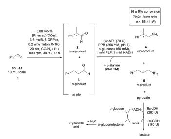
Fig. 5 Chemoenzymatic synthesis of the primary amines 2-phenylpropan-1-amine (4) and 3-phenylpropan-1-amine (5) starting from styrene (1). A 6-DPPon/rhodium-catalysed hydroformylation of styrene (1) applying an aqueous solution utilizing the surfactant Triton X-100 was combined with *Cv*-ATA catalysed enzymatic transamination of the *in situ*-formed aldehydes.
