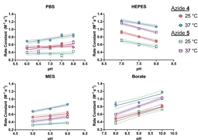
**Fig. 4** The effect of pH on the second-order rate constant ( $k_2$ ,  $[\text{M}^{-1} \text{s}^{-1}]$ ) in selected buffers. Reactions were performed with sulfo DBCO-amine (**1**) and 1-azido-1-deoxy- $\beta$ -D-glucopyranoside (circles, **4**) or 3-azido-L-alanine (squares, **5**) at 25 and 37 °C. Data were fitted to linear regression, with 95% confidence bands of the best-fit line shown as dashed lines. Error bars represent SD ( $n = 3$ ).
