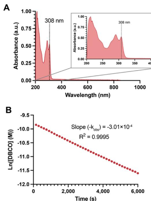
**Fig. 2** (A) UV-Vis spectrum of sulfo DBCO-amine (1) in PBS (pH 7.2). (B) Representative linear graph of the natural log of sulfo DBCO-amine concentration ( $M$ ) vs. time (s) upon the addition of azide 4. Azide 4 = 1-azido-1-deoxy- $\beta$ -D-glucopyranoside, 1 mM. Dotted line represents absorption at 308 nm. Slope ( $-k_{\text{obs}}$ ) and goodness of fit ( $R^2$ ) shown on graph.
