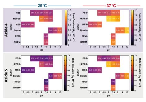
Fig. 3 Heat map of the second-order rate constants of the SPAAC reaction with sulfo DBCO-amine (1). Reactions performed with 1-azido-1-deoxyβ-p-glucopyranoside (4, top) or 3-azido-L-alanine (5, bottom) in various buffers and pH values, at either 25 (left) or 37 °C (right). Values in boxes represent mean rate constants  $(k_2, [M^{-1} s^{-1}])$ .
