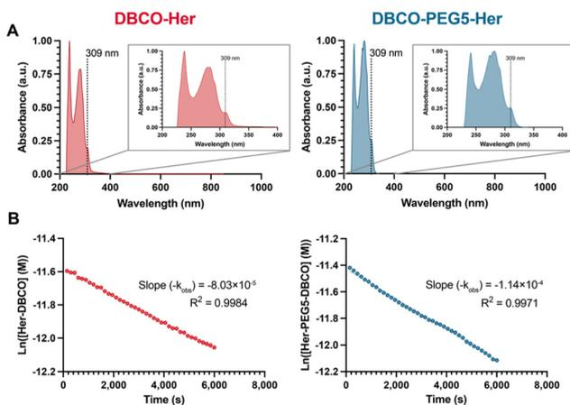
**Fig. 5** (A) UV-Vis spectrum of DBCO-Her conjugates in PBS (pH 7.2). (B) Representative linear graph of the natural log of DBCO-Her concentration ( $M$ ) vs. time (s) upon the addition of azide 4 (1 mM). DBCO-Her (2) is represented in red (left panels) and DBCO-PEG<sub>5</sub>-Her (3) in blue (right panels).
