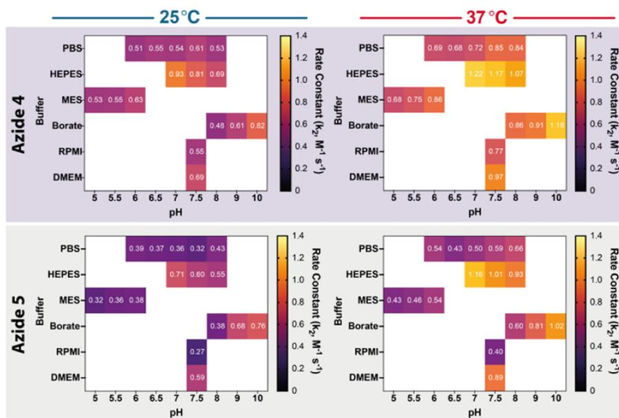
Fig. 3 Heat map of the second-order rate constants of the SPAAC reaction with sulfo DBCO-amine (1). Reactions performed with 1-azido-1-deoxy- $\beta$ -D-glucopyranoside (4, top) or 3-azido-L-alanine (5, bottom) in various buffers and pH values, at either 25 (left) or 37 °C (right). Values in boxes represent mean rate constants ( $k_2$ , [ $\text{M}^{-1} \text{s}^{-1}$ ]).
