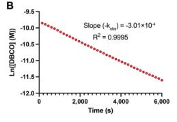
Fig. 2 (A) UV-Vis spectrum of sulfo DBCO-amine (1) in PBS (pH 7.2). (B) Representative linear graph of the natural log of sulfo DBCO-amine concentration (M) vs. time (s) upon the addition of azide 4. Azide 4 = 1-azido-1-deoxy-β-D-glucopyranoside, 1 mM. Dotted line represents absorption at 308 nm. Slope  $(-k_{obs})$  and goodness of fit  $(R^2)$  shown on graph.
