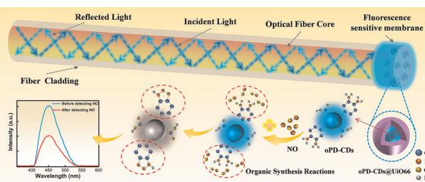
**A new optical fiber sensor based on the CDs@UiO66 complex fluorescence probe for nitric oxide detection**
