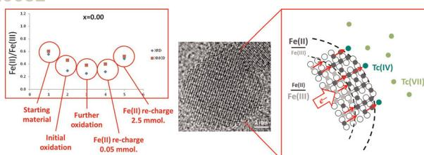
**Oxidation and recharge of reactive structural Fe(II) in titanomagnetite ( $\text{Fe}_{3-x}\text{Ti}_x\text{O}_4$ ) nanoparticles**
