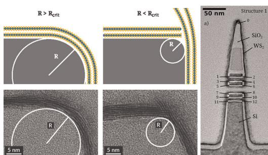
**Conformality limits of 2D WS<sub>2</sub> on 3D nanostructures**
