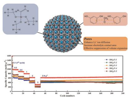
**SiO<sub>x</sub>/C composite spheres as an anode material for high-performance lithium-ion batteries**
