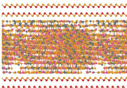
**Simulation of the crystallization process of Ge<sub>2</sub>Sb<sub>2</sub>Te<sub>5</sub> nanoconfined in superlattice geometries for phase change memories**
