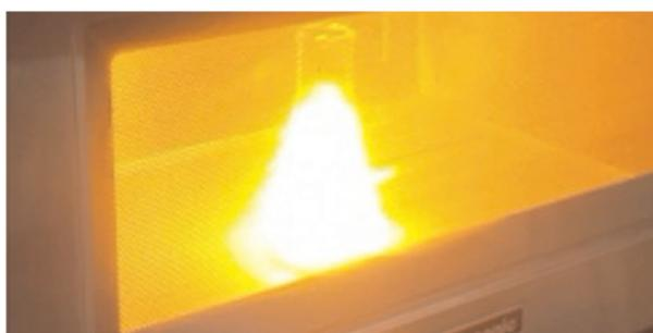
**Intense, self-induced sustainable microwave plasma using carbon nanotubes made from  $\text{CO}_2$**
