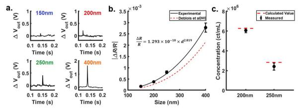
Fig. 3 Validation of the microfluidic resistive pulse device. (a) A typical voltage pulse of 150 nm, 200 nm, 250 nm, and 400 nm gold nanoparticles (note the scaling difference for the 400 nm gold nanoparticles) (b) 150 nm, 200 nm, 250 nm, and 400 nm gold nanoparticles measured  $\Delta R/R$  magnitude and the theoretical  $\Delta R/R$  magnitude calculated from size based on the Deblois's formula.<sup>60</sup> (c) Measured and calculated concentration of 200 nm and 250 nm gold nanoparticles.
