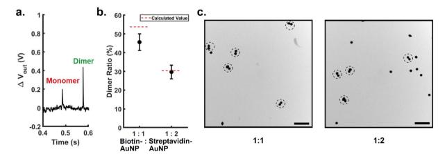
Fig. 4 (a) Typical voltage pulses by a nano-monomer and a nano-dimer. (b) Nano-dimer ratio of Biotin-AuNP: Streptavidin-AuNP at 1:1 and 1:2 mixing ratio. (c) TEM Images of Biotin-AuNP: Streptavidin-AuNP at 1:1 ratio and 1:2 ratio. (The scale bar represents 1.0 μm.)
