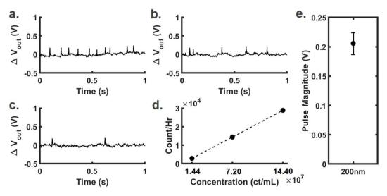
Fig. 2 Typical voltage pulses induced by 200 nm gold nanoparticles passing through the RPS. (a) At  $\sim$ 1.44  $\times$  10<sup>8</sup> ct mL<sup>-1</sup> (b) at  $\sim$ 7.2  $\times$  10<sup>7</sup> ct mL<sup>-1</sup> (c) at  $\sim 1.44 \times 10^7$  ct mL<sup>-1</sup> (d) count rate per hour at  $1.44 \times 10^7$  ct mL<sup>-1</sup>,  $7.2 \times 10^7$  ct mL<sup>-1</sup>, and  $1.44 \times 10^8$  ct mL<sup>-1</sup> (e) voltage pulse magnitude distribution of 200 nm gold nanoparticles.
