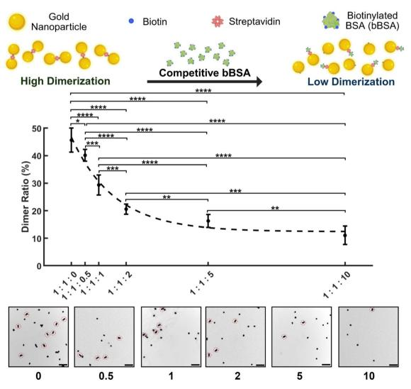
Fig. 5 The measured dimer concentration at different Biotin-AuNPs, Streptavidin-AuNPs and biotinylated BSA mixing ratios (Biotin-AuNP: Streptavidin-AuNP: bBSA) and accompanying TEM images. (The scale bar represents 1.0 μm.) Each error bar represents the standard deviation of 6 tests
