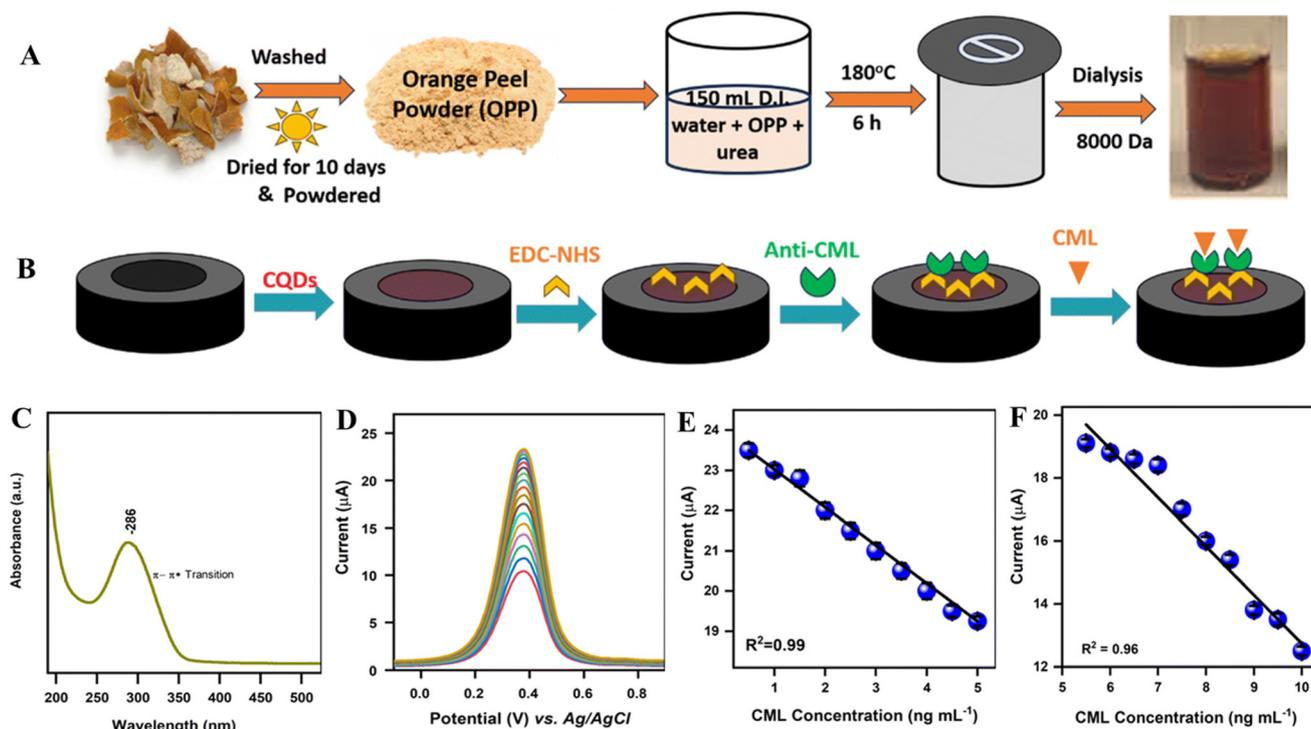
**Fig. 6** (A) Schematic representation for the CQDs; (B) fabrication of the working electrode using CQDs; (C) UV-vis spectrum of CQDs; (D) DPV of the CQDs/anti-CML/EDC-NHS modified GC electrodes in the presence of CML; linear calibration curve for increasing CML concentrations of (E) 0.5–5.0; (F) 5.5–10.0  $\text{ng mL}^{-1}$  with adjusted regression coefficients of  $R^2 = 0.99$  and  $0.96$ , respectively. Reproduced with permission.<sup>91</sup> Copyright 2025, Royal Society of Chemistry.
