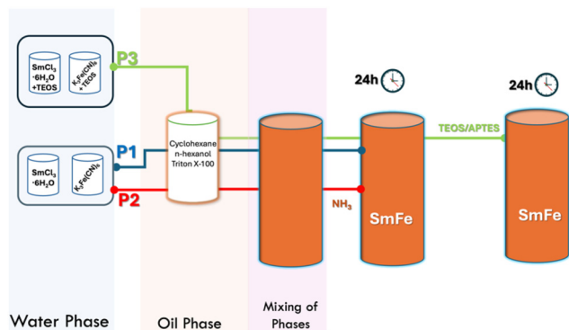
Scheme 1 The experimental protocols P1, P2, and P3 are illustrated schematically, with P1 depicted in navy blue, P2 in red, and P3 in green. The duration of protocols P1 and P2 was 24 hours, while protocol P3 lasted for 48 hours. The experimental protocols P1–P3 depicted in different colours: P1 (blue navy); P2 (red); P3 (green). The ending of protocols P1 and P2 occurred after 24 hours, while for protocol P3, the duration was 48 hours.
