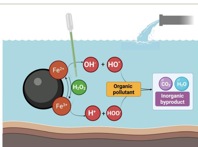
**Fig. 9** Schematic representation of an advanced oxidation process (Fenton reaction). Magnetic nanoparticles (e.g.,  $\text{Fe}^{2+}/\text{Fe}^{3+}$ ) catalyze the decomposition of hydrogen peroxide ( $\text{H}_2\text{O}_2$ ) into reactive oxygen species such as hydroxyl radicals ( $\cdot\text{OH}$  and  $\text{HO}_2\cdot$ ), which degrade organic pollutants into harmless inorganic byproducts like  $\text{CO}_2$  and  $\text{H}_2\text{O}$ . Figure created in Biorender.
