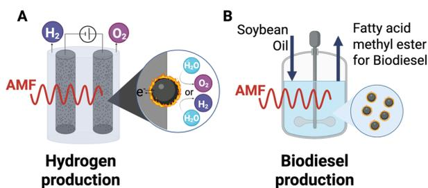
**Fig. 10** Use of MH in green fuel production. (A) In hydrogen production, AMFs can activate magnetic catalysts, enhancing water electrolysis by locally increasing the reaction temperature and improving electron transfer. (B) In biodiesel production, AMF-induced heating of magnetic nanoparticles accelerates the transesterification of oils (e.g., soybean oil) into fatty acid methyl esters, optimizing yield and energy efficiency. Figure created in Biorender.
