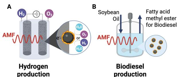
**Fig. 10** Use of MH in green fuel production. (A) In hydrogen production, AMFs can activate magnetic catalysts, enhancing water electrolysis by locally increasing the reaction temperature and improving electron transfer. (B) In biodiesel production, AMF-induced heating of magnetic nanoparticles accelerates the transesterification of oils (e.g., soybean oil) into fatty acid methyl esters, optimizing yield and energy efficiency. Figure created in Biorender.
