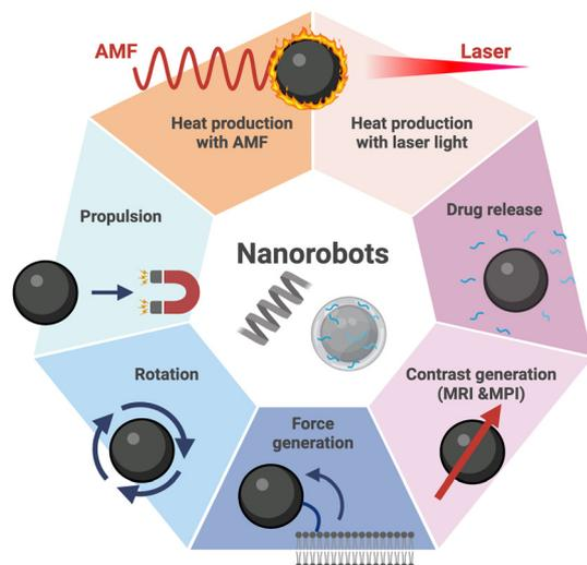
**Fig. 6** Nanorobots are nanoparticles that can perform several tasks, which in the case of magnetic nanoparticles include movement guided by magnetic fields, heat production and other specific activities such as drug delivery or contrast generation in imaging techniques. Figure created in Biorender.
