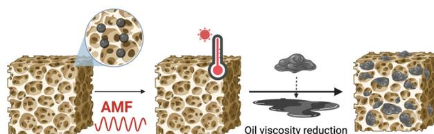
**Fig. 14** Schematic illustration of the design required for enhanced oil recovery (EOR) methods using MNPs (also the so-called “ferrimagnetic sponge”). MH leads to efficient clean-up of viscous crude oil. Figure created in Biorender.
