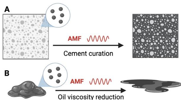
**Fig. 13** Applications of magnetic hyperthermia in construction and oil processing. (A) AMF induces localized heating in magnetic particles embedded in cement mixtures, accelerating curing and enhancing material properties. (B) In oil processing, AMF exposure reduces oil viscosity via magnetic nanoparticle heating, improving flow and facilitating extraction or transport. Figure created in Biorender.
