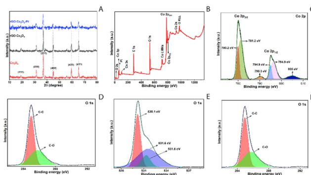
**Fig. 2** Characterization of rGO- $\text{Co}_3\text{O}_4$ -Pt nanocomposites by XRD and XPS. (A) XRD patterns confirm the crystalline structure of  $\text{Co}_3\text{O}_4$  and the incorporation of rGO and Pt nanoparticles into the nanocomposites. (B and C) XPS spectra of Co  $2p_{3/2}$  indicate and Co 2p. (D–F) XPS O 1s spectra.
