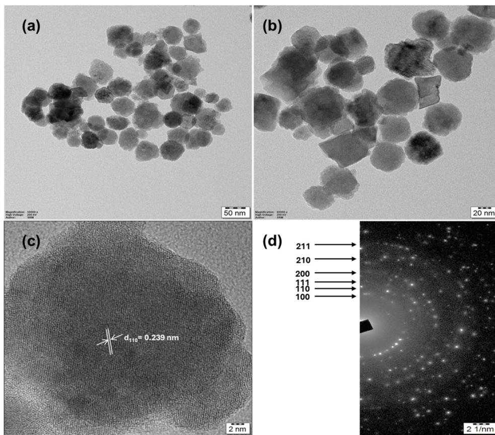
Fig. 9 TEM images of BaTiO<sub>3</sub> synthesized at 30 minutes. (a and b) TEM images at different magnifications; (c) HR-TEM image and (d) selected area electron diffraction (SAED) pattern.
