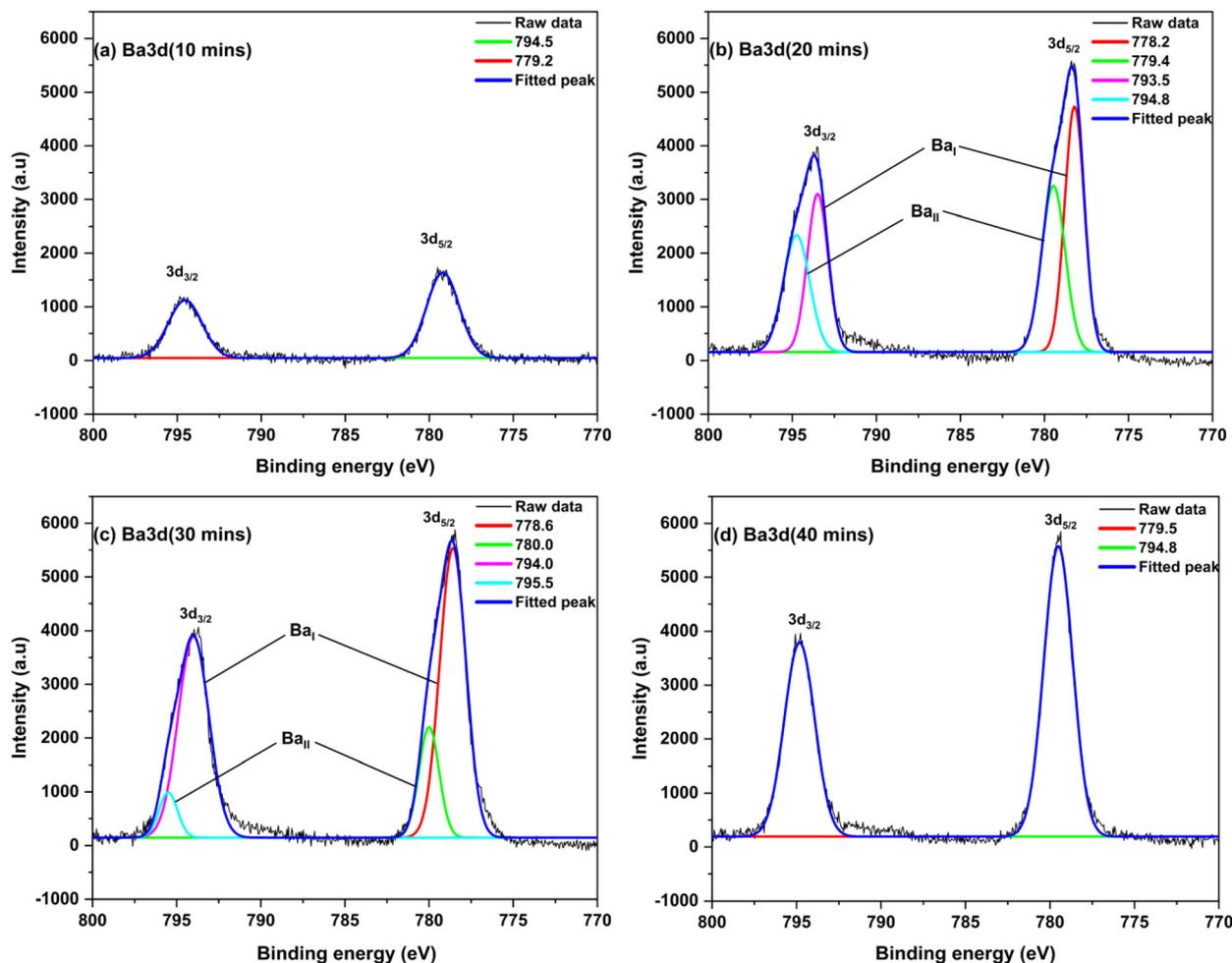
Fig. 11 Deconvoluted spectra of Ba 3d of BaTiO<sub>3</sub> fabricated at (a) 10 minutes, (b) 20 minutes, (c) 30 minutes, and (d) 40 minutes.
