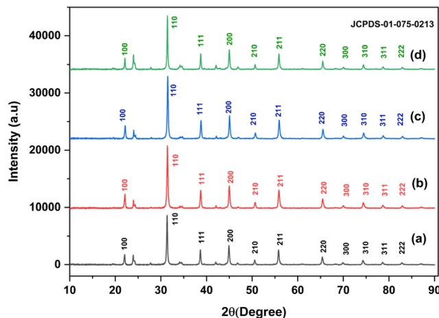
Fig. 2 XRD patterns of the BaTiO<sub>3</sub> samples synthesized using the microwave solvothermal method at 180 °C for (a) 10 minutes, (b) 20 minutes, (c) 30 minutes, and (d) 40 minutes.
