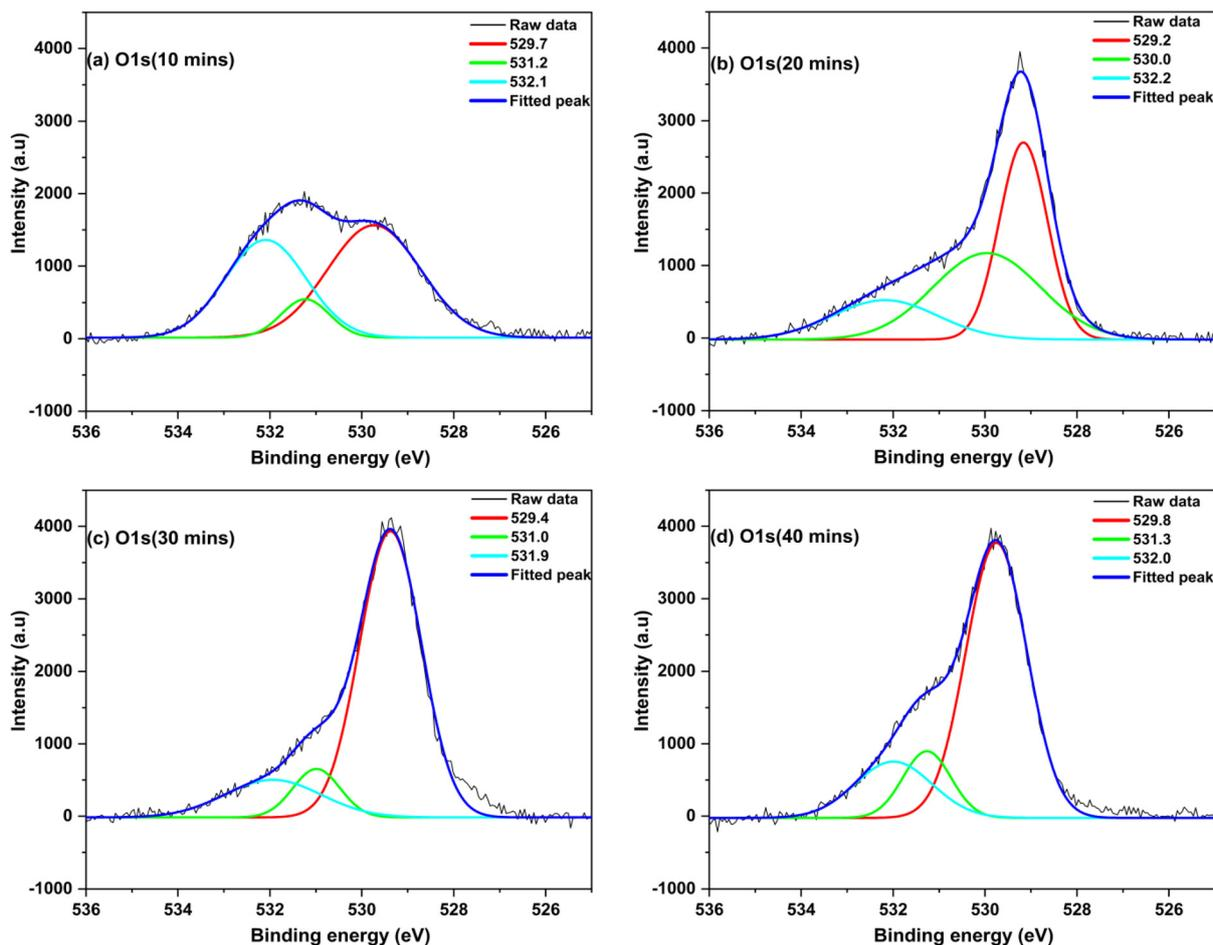
Fig. 12 Deconvoluted XPS spectra of O 1s of BaTiO<sub>3</sub> fabricated at (a) 10 minutes, (b) 20 minutes, (c) 30 minutes, and (d) 40 minutes.
