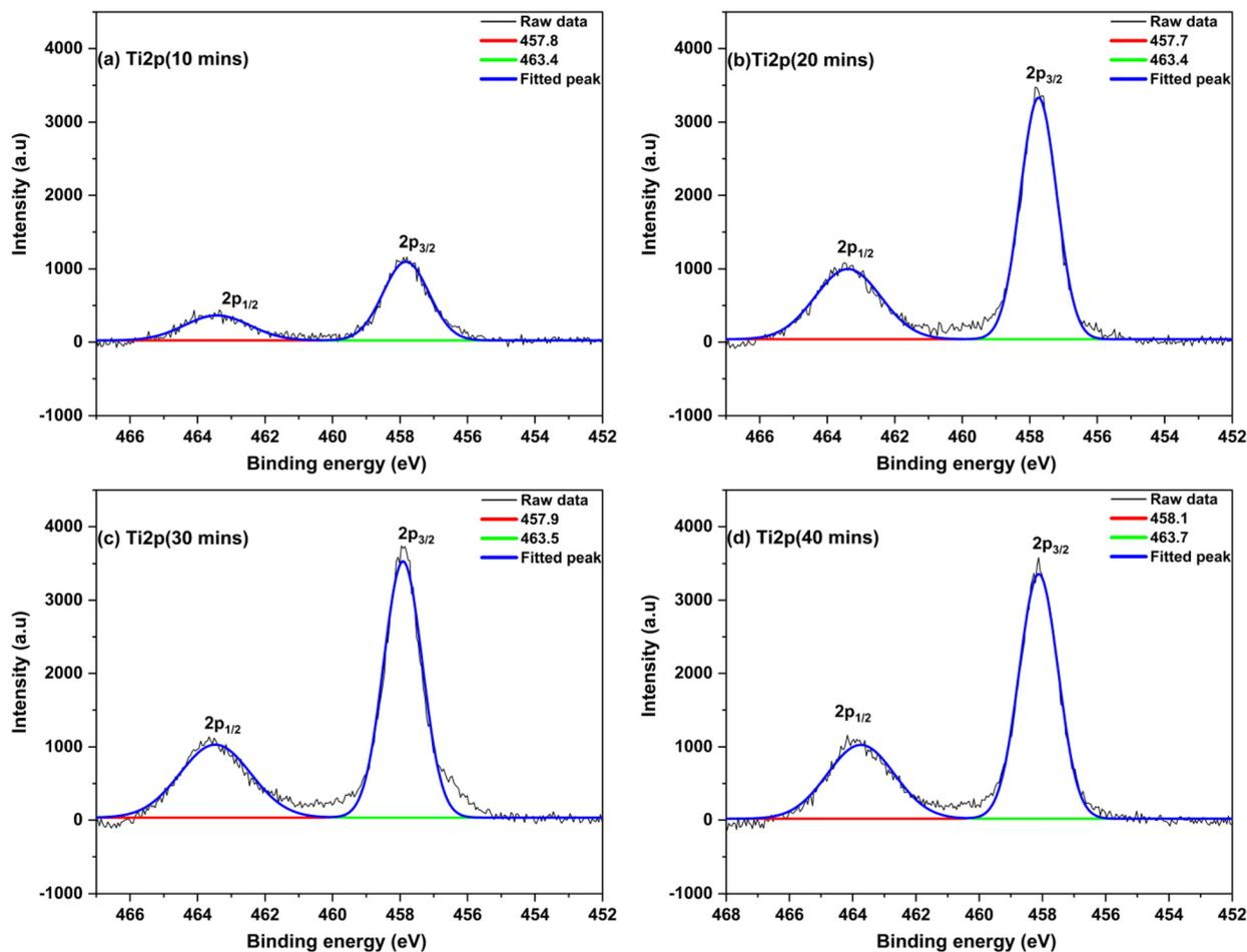
Fig. 13 Deconvoluted XPS spectra of Ti 2p of BaTiO<sub>3</sub> fabricated at (a) 10 minutes, (b) 20 minutes, (c) 30 minutes, and (d) 40 minutes.
