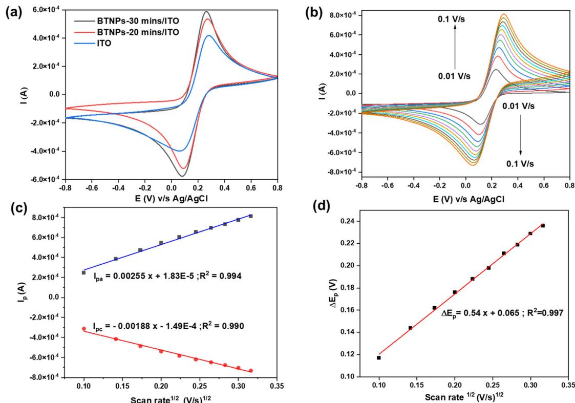
**Fig. 14** (a) CV curves of bare ITO, BTNPs-20/ITO and BTNPs-30/ITO. (b) CV curves of BTNPs-30/ITO at different scan rates. (c) Anodic and cathodic peak current dependence on the square root of the scan rate. (d) Variation of peak-to-peak separation potential with respect to the square root of the scan rate.
