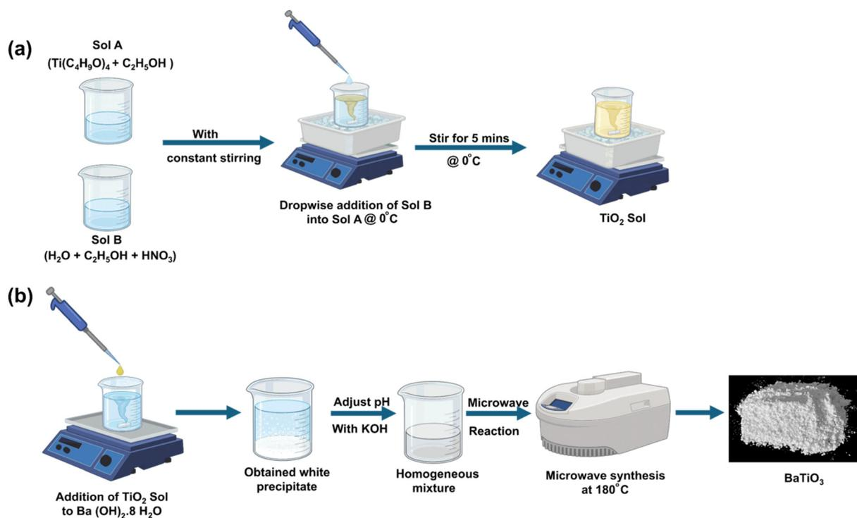
Fig. 1 Schematic representation of BaTiO<sub>3</sub> synthesis. (a) TiO<sub>2</sub> sol formation. (b) BaTiO<sub>3</sub> synthesis.
