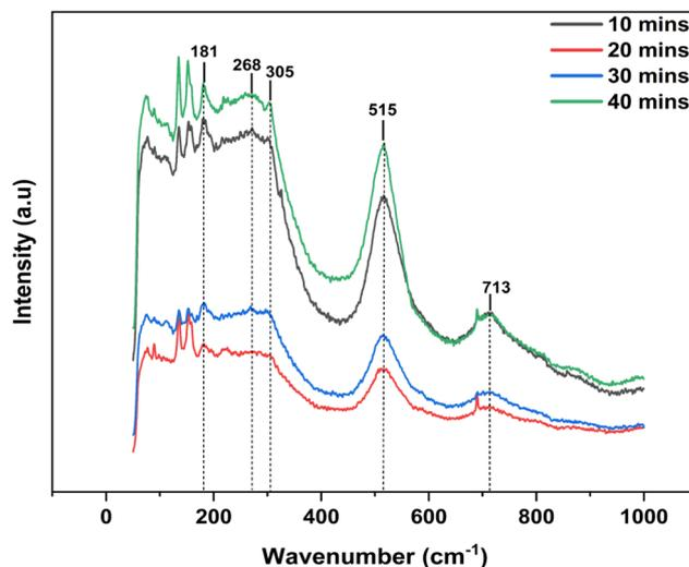
Fig. 6 Raman spectra of BaTiO<sub>3</sub> synthesized at different time durations.
