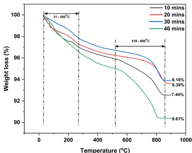
Fig. 5 TGA curves of BaTiO<sub>3</sub> at different synthesis times.
