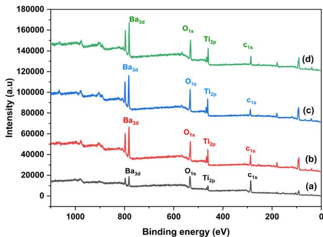
Fig. 10 XPS survey spectra of BaTiO<sub>3</sub> fabricated at (a) 10 minutes, (b) 20 minutes, (c) 30 minutes, and (d) 40 minutes.
