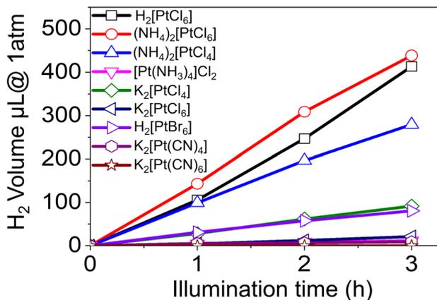
Fig. 2 Photocatalytic H<sub>2</sub> evolution performance of Pt SAs/g-C<sub>3</sub>N<sub>4</sub> prepared with various Pt precursors.
