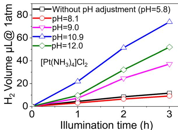
Fig. 3 Photocatalytic H<sub>2</sub> evolution performance of g-C<sub>3</sub>N<sub>4</sub>-supported Pt SAs synthesized from 2 mM [Pt(NH<sub>3</sub>)<sub>4</sub>]Cl<sub>2</sub> with pH adjustment.
