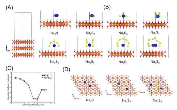
Fig. 2 (A) Clean  $Mg(OH)_2$  surface optimized (B) side views of the surface adsorbate model with the substrates ranging for all sodium polysulfides considered  $(Na_2S_x)$  (x = 1-8) (C) adsorption free energies computed at 0 and 298 K (D) side views of the surface adsorbate models of  $Na_2S_5$  and  $Na_2S_8$ .
