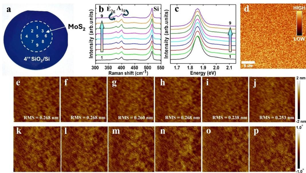
**Fig. 7** (a) Photograph of 2" MoS<sub>2</sub> transferred onto 4" SiO<sub>2</sub>/Si substrate under PMMA/Bi assisted transfer. (b) Raman and (c) PL spectra of MoS<sub>2</sub> film measured from 9 different spots as indicated in (a). (d) Mapping image showing the uniformity of PL intensity captured from MoS<sub>2</sub> (30 × 30 μm). (e)–(j) AFM topography images and (k)–(p) corresponding phase images (10 × 10 μm) of MoS<sub>2</sub> film measured from spots 1 to 6.
