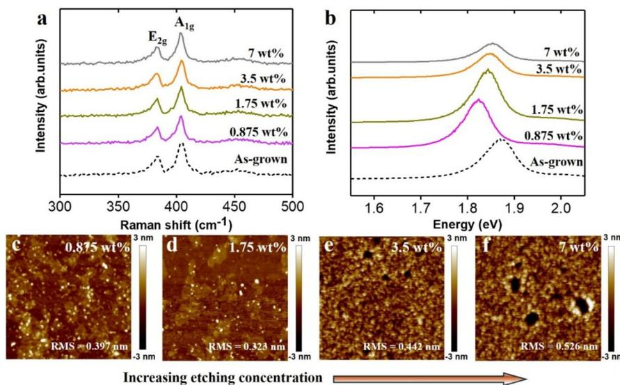
**Fig. 3** (a) Raman spectra, (b) PL spectra and (c)–(f) AFM topography images ( $1 \times 1 \mu\text{m}$ ) of PMMA/Bi assisted transferred  $\text{MoS}_2$ . PMMA were dissolved in hot acetone for 2 hours, followed by the Bi etching process in nitric acid solution under various concentration (0.875 wt%, 1.75 wt%, 3.5 wt% and 7 wt%) for 30 minutes. Raman and PL properties of the as-grown  $\text{MoS}_2$  are indicated as a reference (dashed curve in (a) and (b)).
