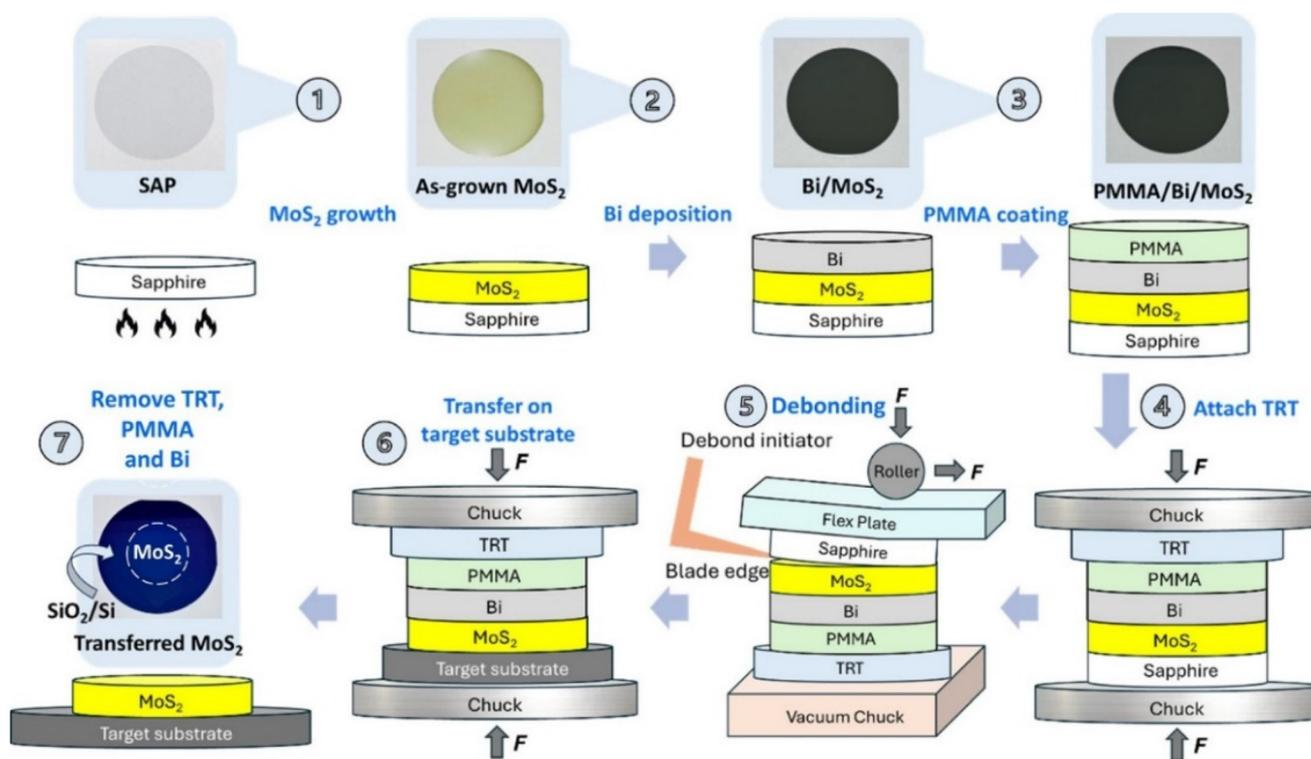
Fig. 1 Schematic drawings and photographs of samples in PMMA/Bi assisted transfer process for monolayer MoS<sub>2</sub>.
