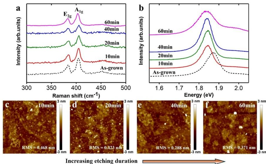
**Fig. 4** (a) Raman spectra, (b) PL spectra and (c)–(f) AFM topography images ( $1 \times 1 \mu\text{m}$ ) of PMMA/Bi assisted transferred MoS<sub>2</sub>. PMMA were dissolved in hot acetone for 2 hours, followed by the Bi etching process in 1.75 wt% nitric acid solution under various duration (10, 20, 40 and 60 minutes). Raman and PL properties of the as-grown MoS<sub>2</sub> are indicated as a reference (dashed curve in (a) and (b)).
