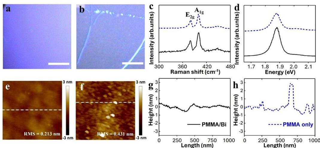
**Fig. 2** (a and b) Optical microscopy images with scale bar of 10  $\mu\text{m}$ . (c) Raman spectra, (d) PL spectra, (e and f) AFM topography images ( $1 \times 1 \mu\text{m}$ ), and (g and h) cross-sectional profiles taken along the location marked in (e and f), of monolayer  $\text{MoS}_2$  after (a, c–e and g) PMMA/Bi assisted transfer and (b–d, f and h) PMMA-only assisted transfer.
