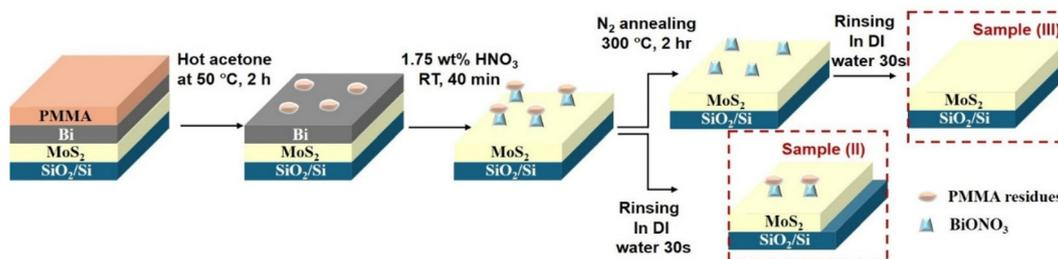
**Fig. 6** Schematic drawings depict the process flow during the removal of PMMA/Bi support layer from MoS<sub>2</sub>. After DI water rinsing, both samples (II) and (III) were subsequently dried using N<sub>2</sub> blow-drying.
