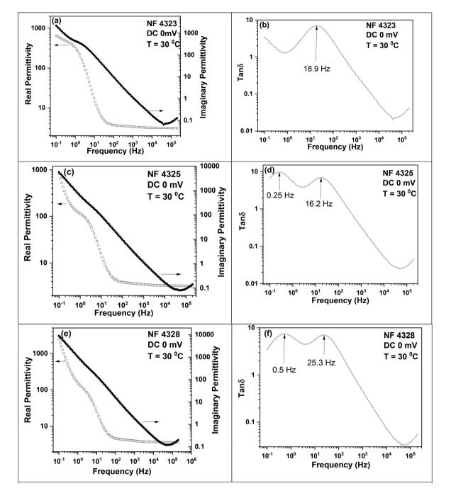
Fig. 3 Real and imaginary permittivities measured at 30 °C under no bias conditions for the (a) NF 4323, (c) NF 4325, and (e) NF 4328 magnetic fluids. Dissipation factor for the (b) NF 4323, (d) NF 4325, and (f) NF 4328 magnetic fluids.
