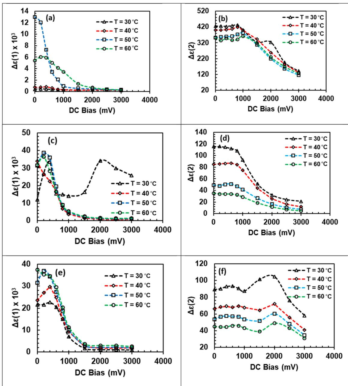
Fig. 8  $\Delta\epsilon_1$  values for the (a) NF 4323 fluid, (c) NF 4325 fluid, and (e) NF 4328 and  $\Delta\epsilon_2$  values for the (b) NF 4323 fluid, (d) NF 4325 fluid, and (f) NF 4328 fluid as a function of DC bias voltages.
