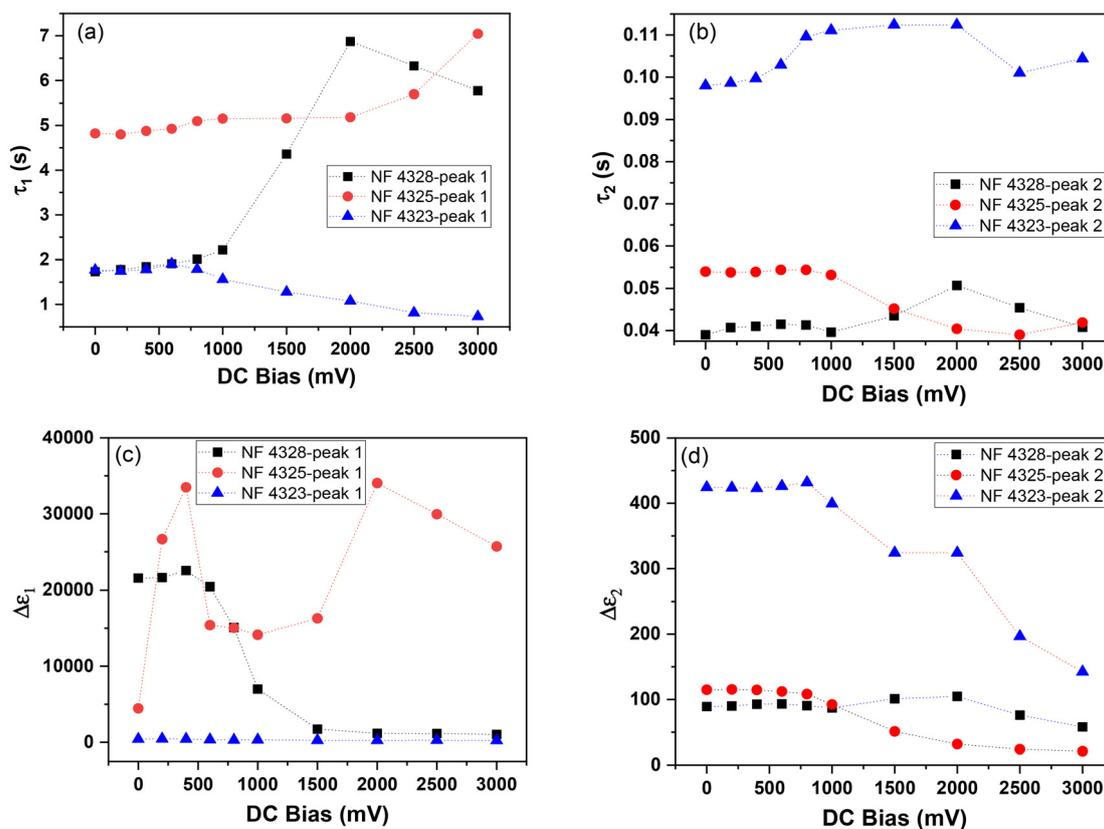
Fig. 5 Relaxation time for (a) the low-frequency peak and (b) the high-frequency peak and variation in (c) the  $\Delta\varepsilon_1$  and (d)  $\Delta\varepsilon_2$  values as a function of DC bias voltages for all three samples.
