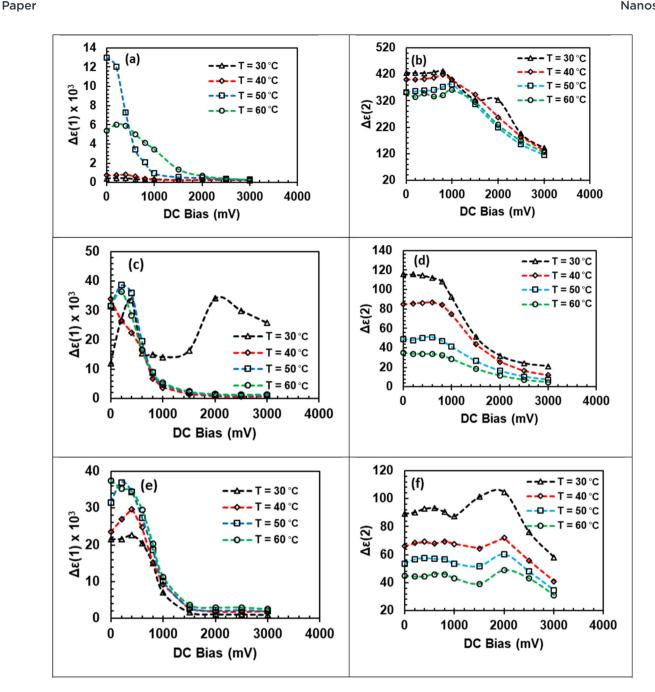
Fig. 8  $\Delta \varepsilon_1$  values for the (a) NF 4323 fluid, (c) NF 4325 fluid, and (e) NF 4328 and  $\Delta \varepsilon_2$  values for the (b) NF 4323 fluid, (d) NF 4325 fluid, and (f) NF 4328 fluid as a function of DC bias voltages.
