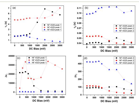
Fig. 5 Relaxation time for (a) the low-frequency peak and (b) the high-frequency peak and variation in (c) the  $\Delta \varepsilon_1$  and (d)  $\Delta \varepsilon_2$  values as a function of DC bias voltages for all three samples.
