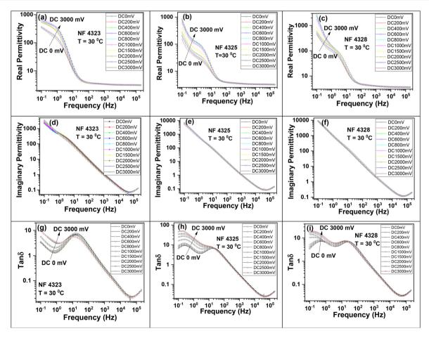
Fig. 4 Real permittivity (a)–(c), imaginary permittivity (d)–(f), and dissipation factor (q)–(i) as a function of frequency under different bias conditions at 30 °C for the NF 4323 magnetic fluid, NF 4325 magnetic fluid, and NF 4328 magnetic fluid, respectively.
