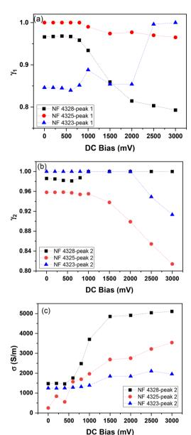
Fig. 6 Variation in the (a)  $\gamma_1$  and (b)  $\gamma_2$  values and (c) conductivity as a function of DC bias voltages for all three samples.
