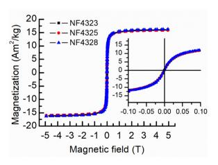
**Fig. 1** The studied magnetic fluids' isothermal (298 K) magnetisation curves. The inset shows the superparamagnetic fluctuations of the magnetic moments in the absence of a magnetic field.
