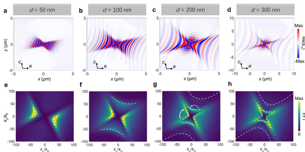
**Fig. 3** The asymmetric directional propagation of hyperbolic shear polaritons in bGO slab. (a)–(d) Numerical field distribution, that is, real part of  $E_z$ , ( $\text{Re}(E_z)$ ), of the dipole-launched polaritons above the surface at  $\omega = 718\text{ cm}^{-1}$ . (e)–(h) The corresponding fast Fourier transform (FFT). The red and white dashed curves represent analytical dispersion of the fundamental and higher-order modes, respectively.
