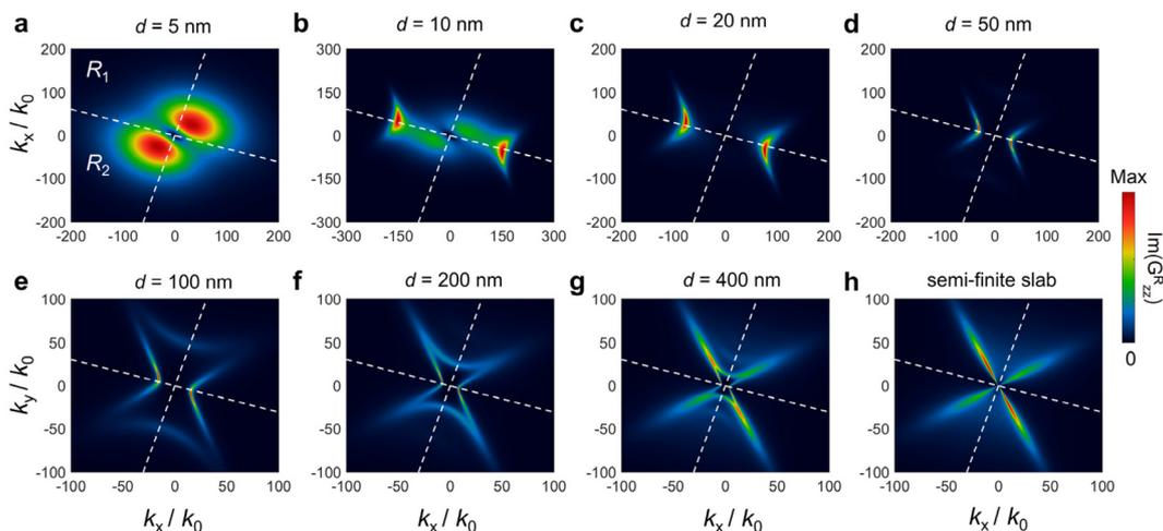
**Fig. 6** The distribution of the imaginary part of reflected Green's function in momentum space,  $\text{Im}(G_{zz}^R(k_x, k_y))$  for different thicknesses of bGO slab. The frequency is fixed to  $718 \text{ cm}^{-1}$ . The white dashed lines are parallel to the effective optic axes, dividing the  $k$  space into four quadrants.
