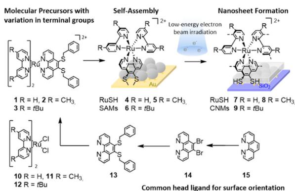
**Fig. 1** Preparation of RuSH CNMs **7–9** by self-assembly of Ru(II) precursors **1**, **2** or **3** into the respective SAMs **4–6** and subsequent low-energy electron beam irradiation. Terminal groups of the complexes can be varied due to the modularity of the precursors **10**, **11** and **12**. The thiolated phenanthroline **13** serves as a common head group and enforces the attachment of the phenanthroline ligand on the Au surface.
